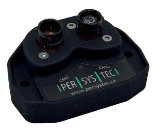
CANBG2 Dual channel CAN bus gateway forwards CAN data from one channel to another. It is offering fast processing solution to bridge between two isolated CAN buses where complexity and lengths of the buses are critical. Programmable hardware filters give the opportunity to either forward all traffic or select packets with specific arbitration ID.
